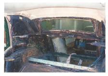
The rear window frame was totally rotten, which meant making an exact replica
