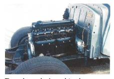
The engine received new piston rings, re-ground valves and other essential work
