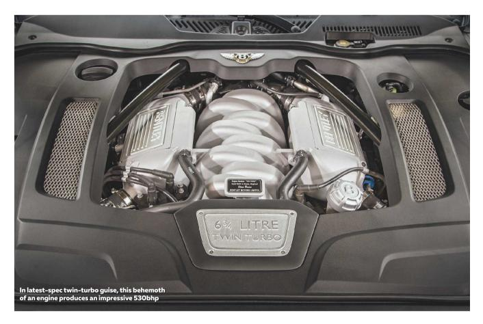
its capacity grew to 6.75 litres by increasing the stroke. In six-and-three-quarter guise, the V8 went on to power every subsequent Rolls-Royce and Bentley (until more recent years), with a major change coming in 1980 via the introduction of Bosch K-Jetronic fuel-injection in order to help meet emissions regulations.
