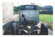
The entire front end was removed for bodywork repairs with the engine out
