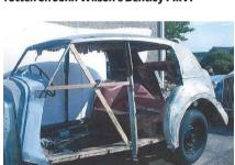
The bodyshell was braced to ensure there were no problems with distortion
